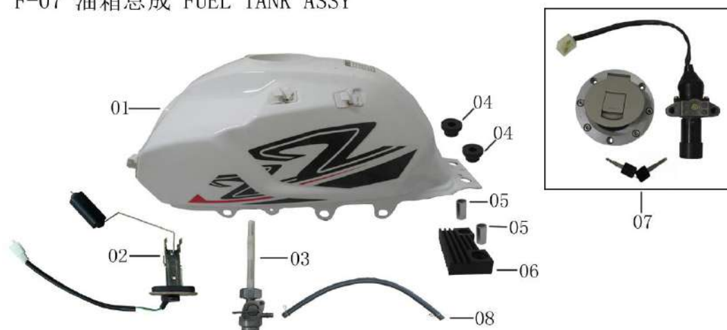
F-07 油箱总成 FUEL TANK ASSY
